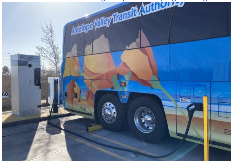
Exhibit C.1.1 AVTA bus using a depot-based plug-in charger
