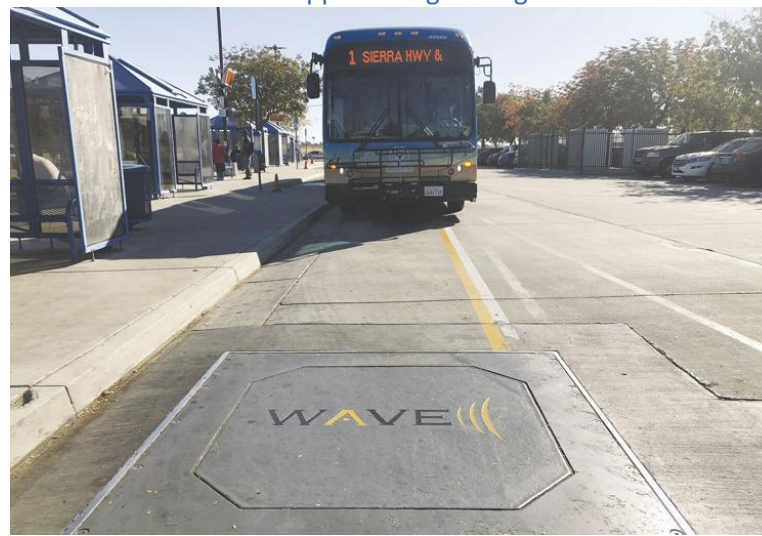
Exhibit C.1.2 AVTA bus approaching an in-ground inductive charger
