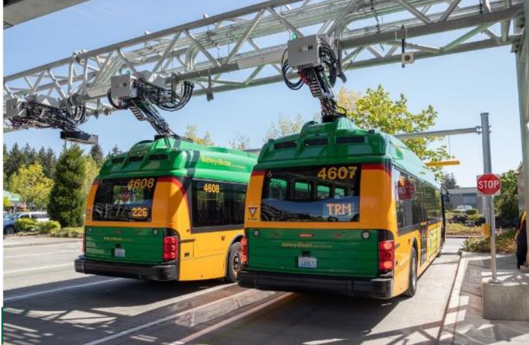
Exhibit C.1.5 Example of gantry-based overhead pantograph charger
