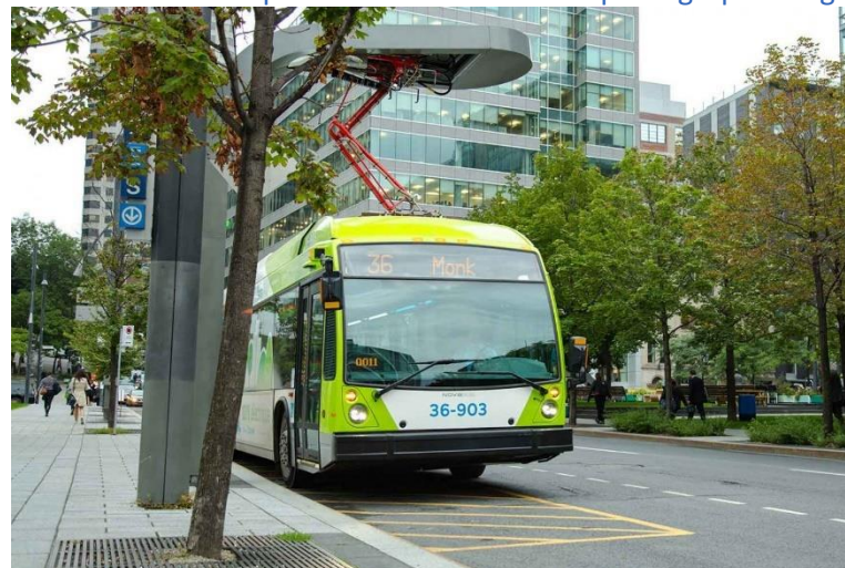
Exhibit C.1.4 Example of on-route overhead pantograph charger
